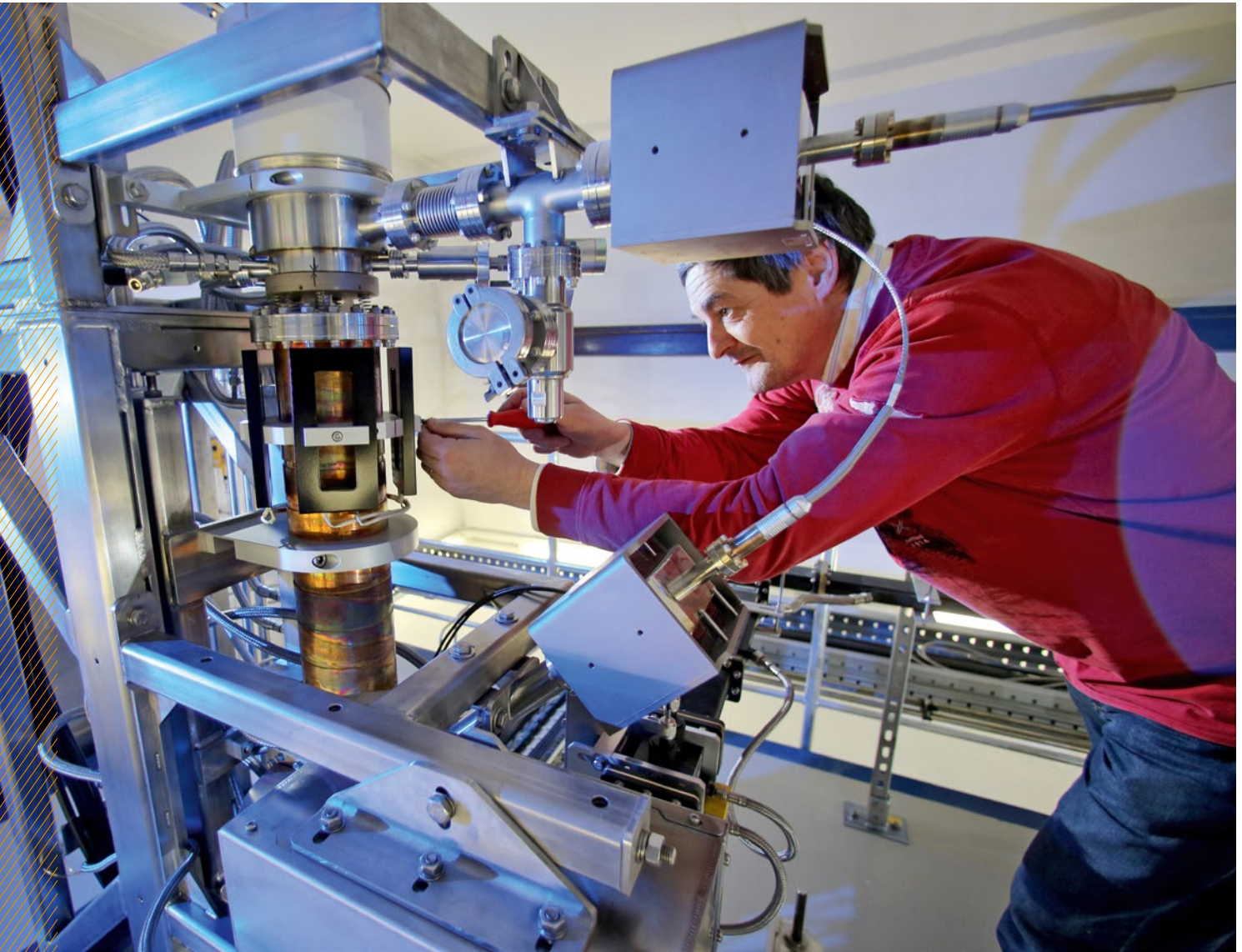
Wolfgang Knolle, research assistant, at the 10 MeV electron accelerator in the Hertz Electron Beam Laboratory at the IOM. Photo: Jan Woitas
