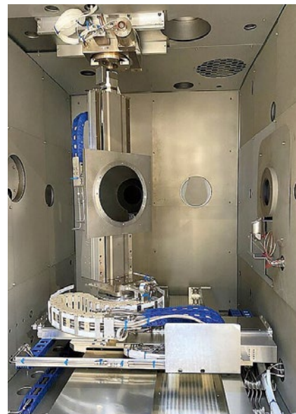
View into the process chamber of the universal diagnostic platform for reactive ion beam processes. Photo: Peter Birtel
