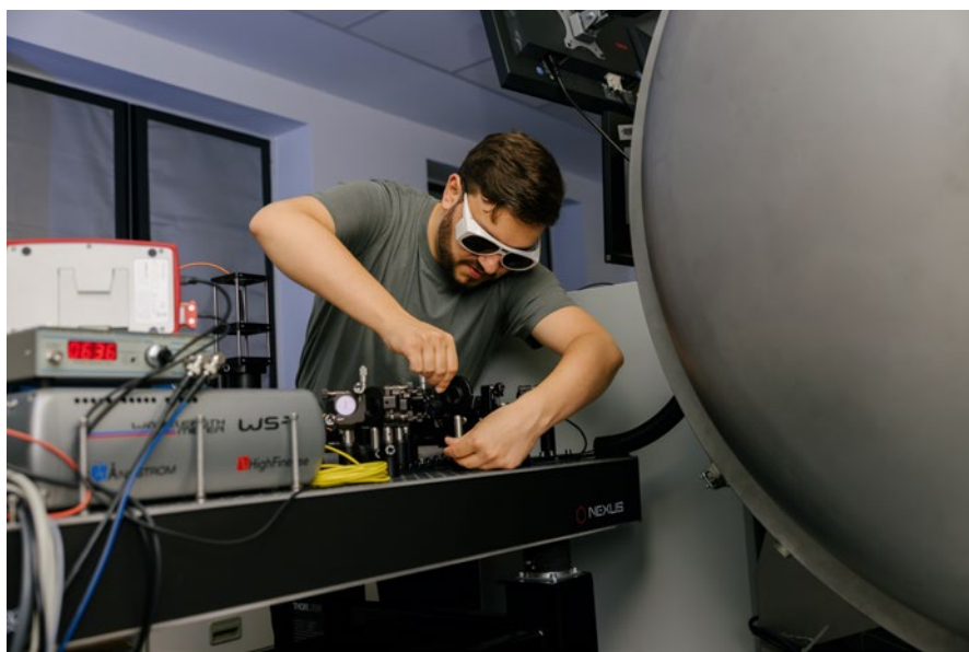
Lukas Pietzonka, research assistant, adjusting the optical components for laser-induced fluorescence spectroscopy. Photo: Erik Kazak
