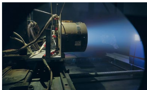
Left: Laser spectroscopic investigation of a xenon-powered RIT-10 EVO (provided by ArianeGroup GmbH) in a vacuum chamber at IOM Leipzig. (Photo: Lukas Pietzonka) Right: IOM expert Dr. Daniel Spemann
